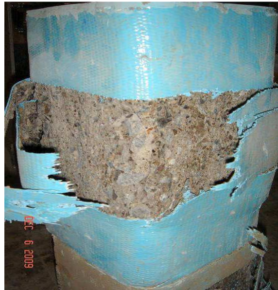
Fig 17 GFRP wrapped square prism with rounded edges 195 x 195 mm in size
