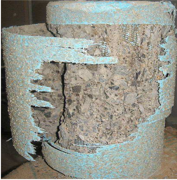
Fig 14 GFRP wrapped cylinder 150 mm in diameter failure due to tearing of fibers
