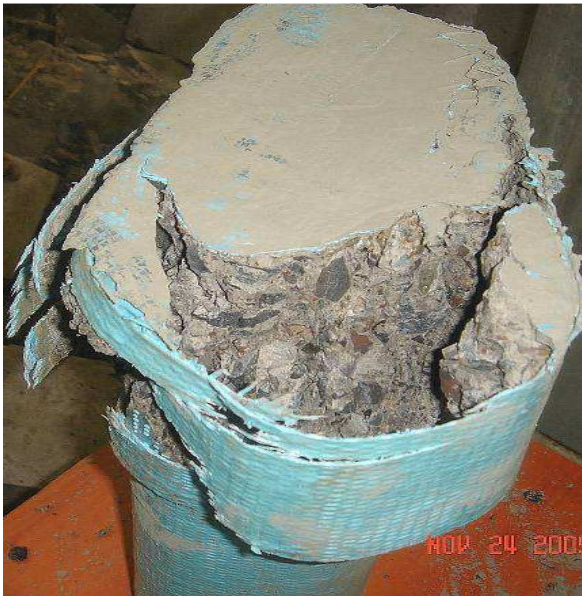
Fig 16 GFRP wrapped square prism with rounded edges 100 x 180 mm in size
